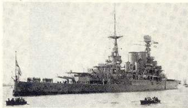
A view of HMS Repulse in the 1920s before the small AA guns and hangers were fitted, and with flying-off platform on the after-turret.
