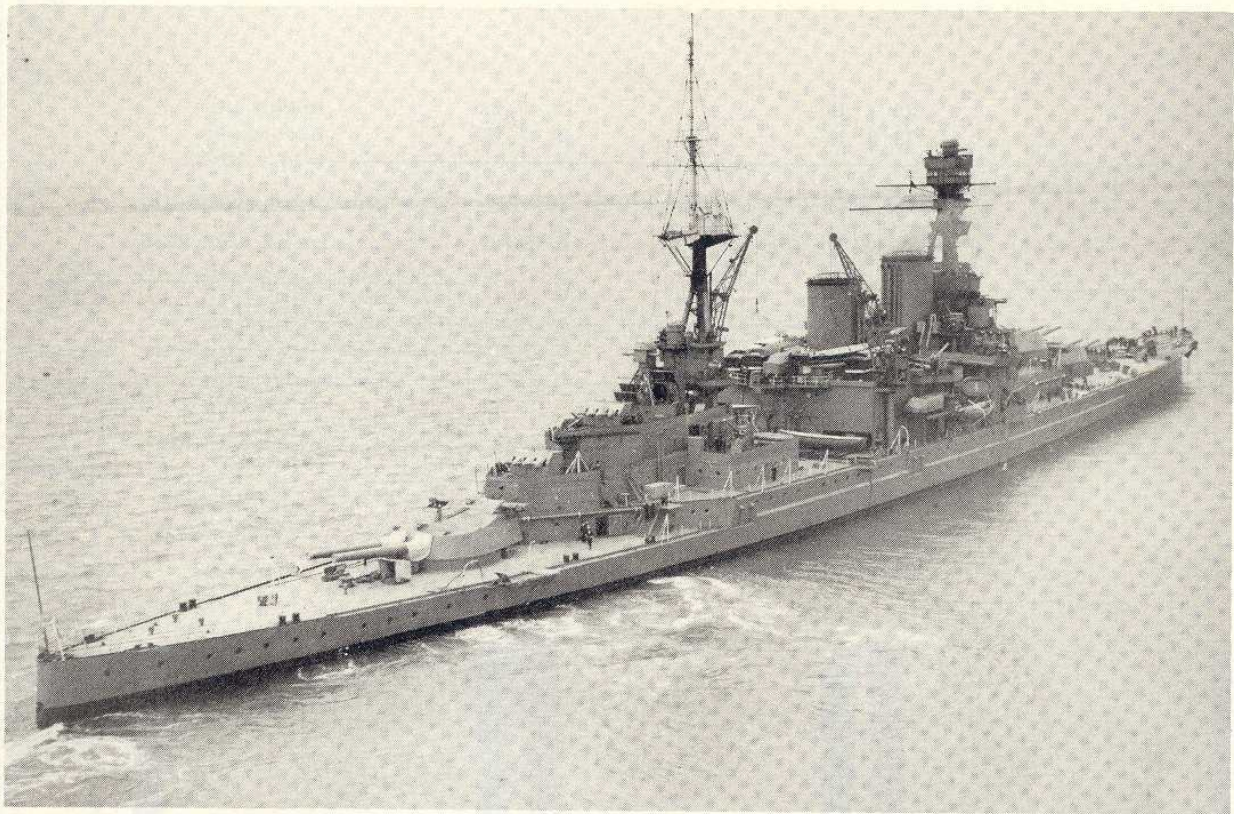
HMS Repulse about to anchor, is manoeuvring with its screws; the cranes being topped up preparatory to hoisting boats. Picture dates from around 1939-40.
