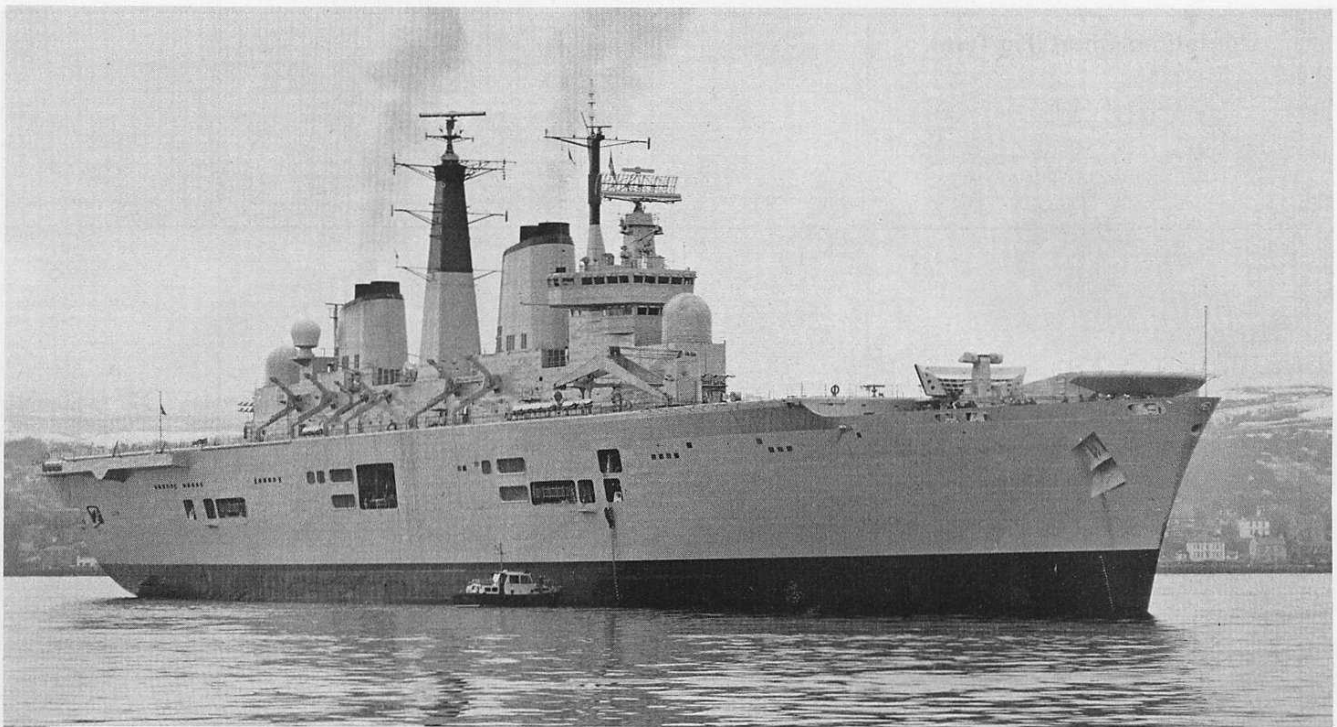
Backbone of the hard pressed ASW task force deployments, the Through Deck Cruiser, is equipped with 5 Harriers and 9 Sea King ASW Helicopters, and the World's most advanced ASW warfare kit, including a new type of sensor which can detect the smallest particles of radio-activity at great depths, ie The radio-active 'hot' water, used for reactor cooling on nuclear powered submarines. Seen here is the first ship of the class, HMS Invincible, which can stand up to almost anything the Soviet Navy can throw at her, with the exception of British Government Policy! Her major vulnerability is a successive attack of Politicians (RN 11161A|2).
