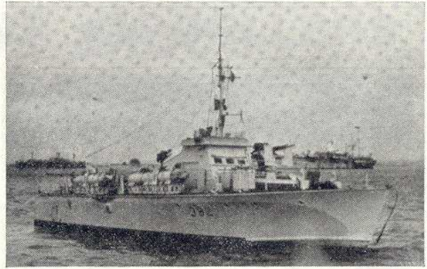
Vosper MTB number 382. Note canvas covers over torpedo tubes. Can any reader give us any information on this particular ship?
