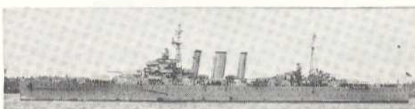
Top: Cruiser Shropshire with original arrangement of one HACS Mk I director aft (abaft crane). Above: HMAS Australia in 1946 as modified with 'ended' HACS arrangement.
