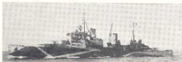
Above: Uganda in 1943 with 'ended-sided' director layout. Right: Coventry as an AA cruiser in 1937 with Mk III director on Spotting Top.
