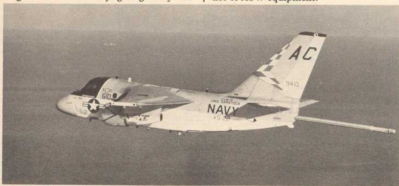
The United States Navy S-3A Viking, is one of the most advanced Carrier Borne ASW Hunter Killers available today. It has on board the most sophisticated array of avionics ever developed for a tactical aircraft, including a large on-board digital computer. The probe which can be seen extended from the tail in this view, carries a set of various types of sensor including the MAD, and Linescan pickups (Lockheed Aircraft).
