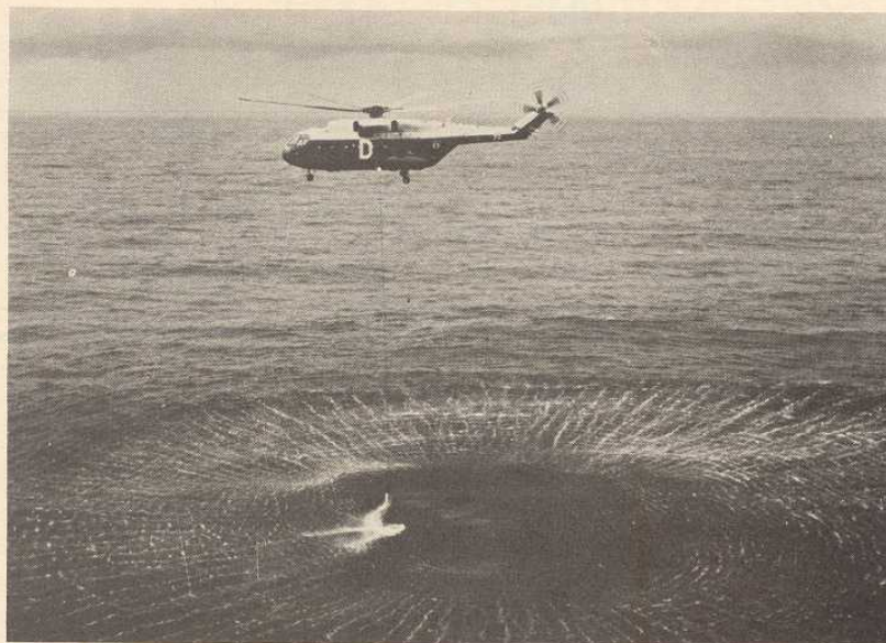
A French Navy SA-321G Super Frelon operates a dunking sonar search off the Atlantic coast.
