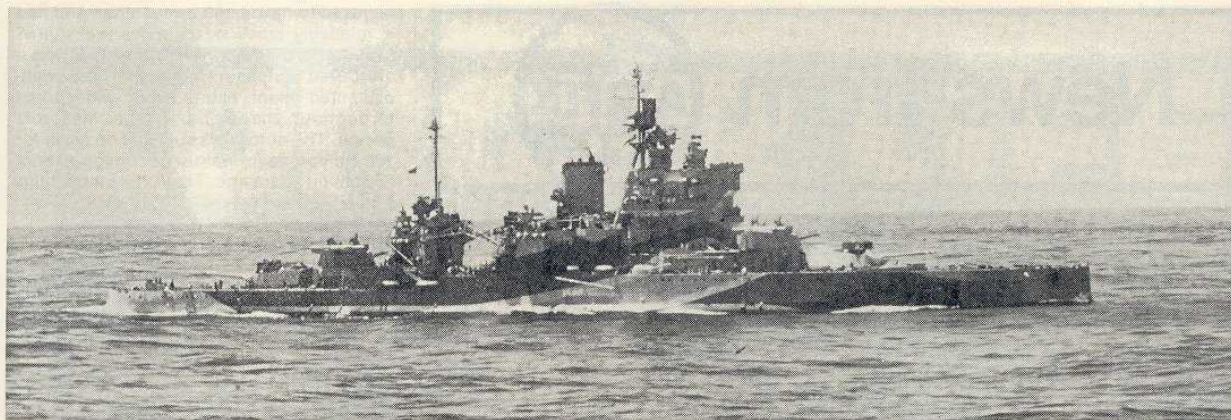
HMS Valiant in the 1943-44 period as depicted in the author's drawing (B). The drawing shows port side camouflage and this view shows the starboard pattern (IWM-A21712).
