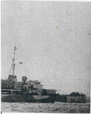
HMS JAMAICA in World War 2, when she still carried a fourth 6-inch turret in X position. At this period she had two cranes and carried her motor-boats on the after superstructure. (Photo by Real Photographs Co Ltd.)
