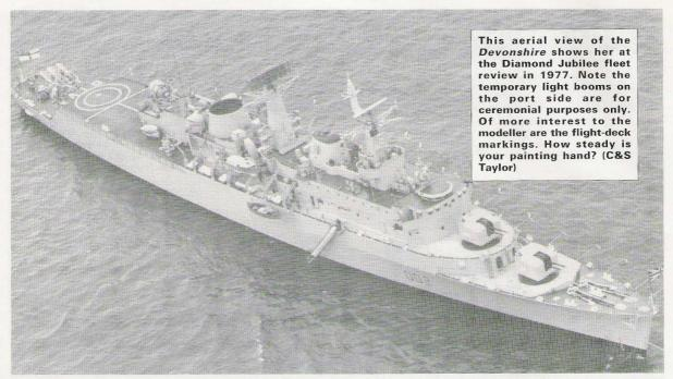
was completed by two turrets forward, each mounting a pair of 4.5in guns and a pair of quadruple Shorts Seacat GWS 22 air defence missile launchers, abreast of the hangar aft. All the ships embarked a Westland Wessex HAS. 1 anti-submarine helicopter (depicted in the kit), later replaced by the Wessex HAS. 3 version.
