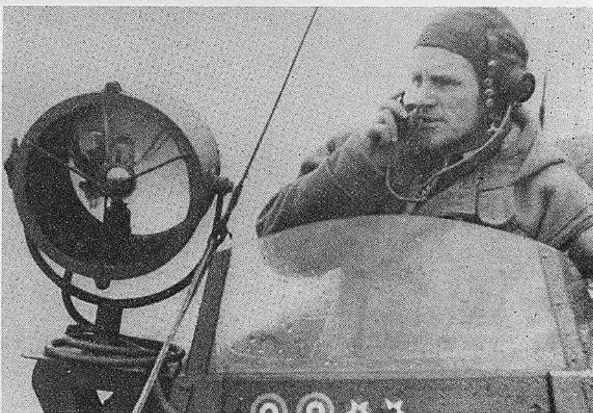
Above: There is a vast amount of information to be gleaned from this photograph of Flying Officer G. Lockwood, skipper of HSL 156 when based at Newhaven. The searchlight is shown on its small platform alongside the hatch. The skipper wears a duffel coat and an aircrew type flying helmet with earphones. He is talking here on R/T with base or an aircraft. On the coaming are small RAF roundels and USAAF stars to indicate successful recoveries.
