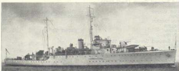
The name-ship of the 'Egret' class exhibits the same characteristics as Bittern but has the fourth 4 inch mounting on the quarterdeck. Notice the searchlight and machine gun platforms in this 1938 photograph (Wright and Logan).
