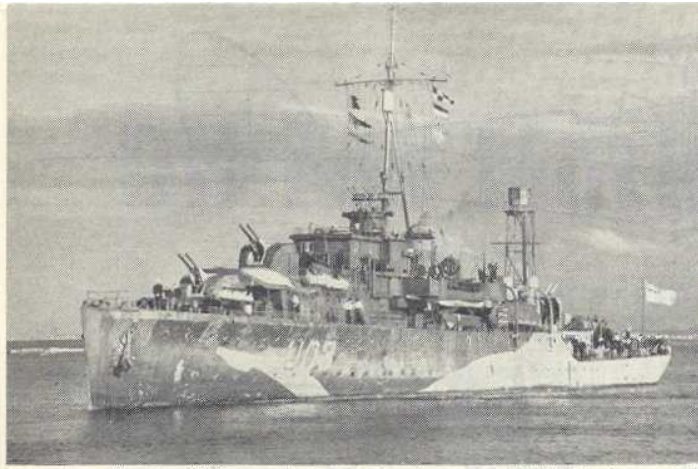
Erne in 1943 warpaint, returning from patrol. She has four single Oerlikons, the quarterdeck pom-pom and the familiar Radar Type 272 on a tall and somewhat fragile-looking pylon (Imperial War Museum).
