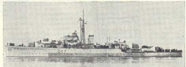
Black Swan in 1945. She has twin Oerlikons in the bridge wings, 'sided' single Oerlikons on a gundeck at the break of the fo'c'sle deck and a quad pom-pom on the quarterdeck. Notice the absence of a close range gundeck immediately abaft the funnel (Imperial War Museum).
