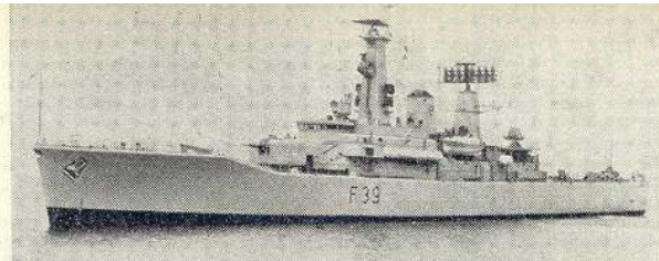
Above: HMS Naiad with Seacat launcher aft (Picture from 'Navy News' postcard series—prints available at 1s 6d each from 'Navy News', RN Barracks, Portsmouth, Hants).
