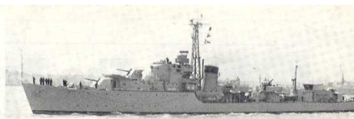
Above: HMS Wizard post-war with the single small HA director, two single Bofors abaft the funnel with a twin Bofors mount amidships.
