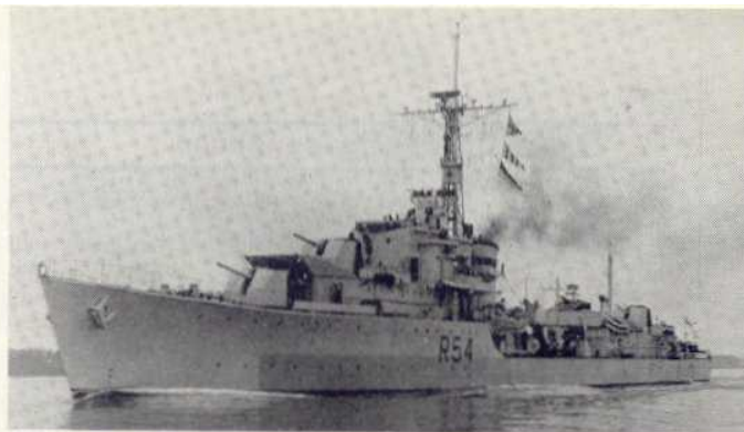
Above: HMS Zodiac with typical late fittings—lattice masts, twin Bofors amidships, a single director, and 4.5 inch guns (Imperial War Museum).
