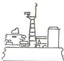
1955 modification showing lattice mast and radar
