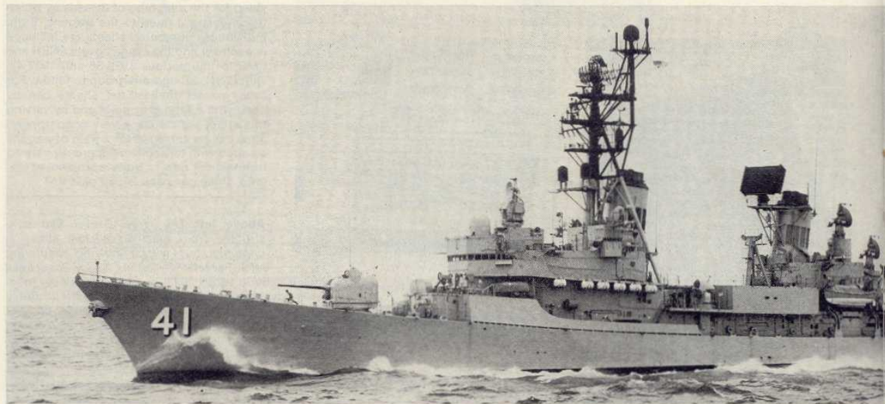
Above HMS Hobart entering Sydney harbour. Note the Ikara missile, deck lockers and foremast detail. Below HMAS Brisbane at sea showing a view of the Ikara deckhouse and launcher (Photos RAN Official via Paul Beaver).
