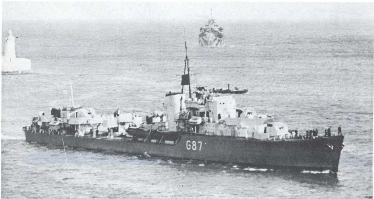
The AA destroyer Lance showing the distinctive twin 4 inch mounts, quite different from the big 4.7 inch gun houses (IWM-A7266).
