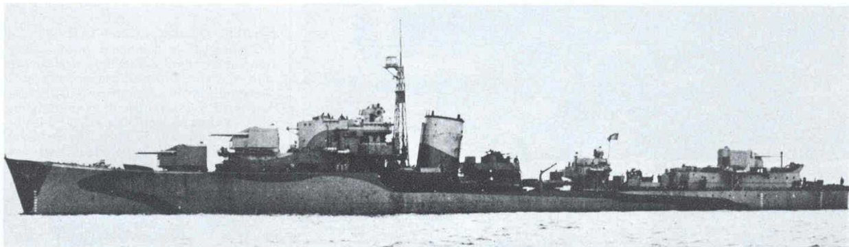
The 'M' class Leader Milne . Note long deckhouse, lattice mast, Carley rafts painted in red/yellow quarters (IWM-A19902).
