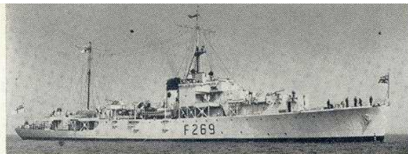
The last 'River' class to be actively employed in the Royal Navy was HMS Meon. Notice the revised gun armament, exclusively of close-range weapons, and particularly the special Oerlikon sponson above the post-war pendant number. As an HQ ship for landing craft, she had an extensive radio system, and wore the 'Combined Ops' badge on her funnel beneath the 'leaders' band.
