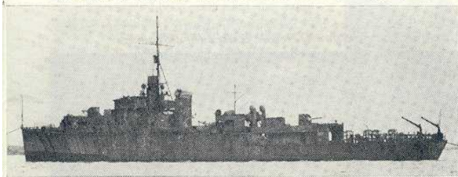
Notice the prominent minesweeping davits on the quarters of Ness, and the extensive depth charge stowages. The photograph dates from June 1950, when her working days were over. (P. A. Vicary).
