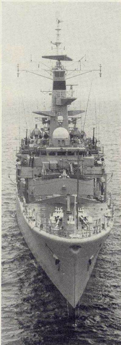
A fine bow shot of Leander showing the Ikara well and superstructure, plus the thimble director.
