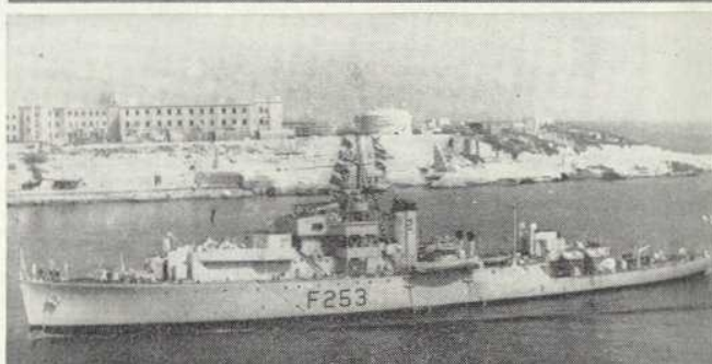
Top: HMS Test off Portsmouth in 1952, when she was in reserve. Notice the 'boxed in' bridge wings, the radar lantern on the bridge and the HF/DF aerial on the fore topmast (Wright & Logan). Above: HMS Helmsdale entering Malta in 1953, with Hedgehog and double Squid but with the earlier D/C armament removed (A. & J. Pavia).
