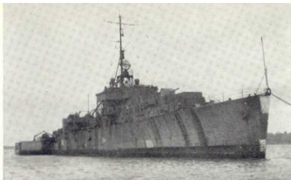
Kale, in reserve in 1950, looks rust-streaked and neglected, but the strong workman-like hull is still evident. Notice the Radar Type 277 aerial on the bridge pylon.
