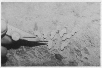
The air intake ducts (parts 61 and 62) can be thinned down to a neater appearance using a sharp knife.
