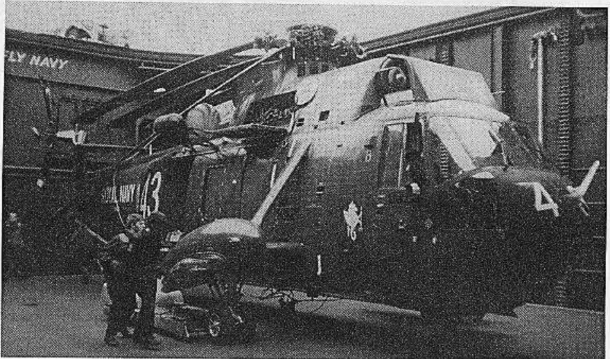
Right: All set to go up on the after lift is one of the retro-fitted Mark 2 Sea Kings. To save space and hence allow more helicopters to be carried, the Sea King, like the Wessex has folding rotors and tail unit. Below: Flying operations on the flight deck of Bulwark as she steams off the Scottish Coast. So far, during her 'new' career, Bulwark has managed to complete all her tasks on or even before time ( HMS Bulwark ).
