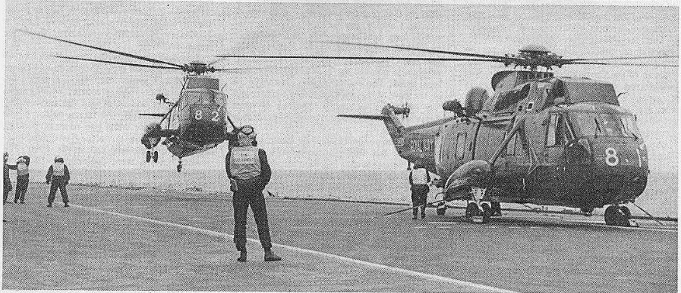
Right: All set to go up on the after lift is one of the retro-fitted Mark 2 Sea Kings. To save space and hence allow more helicopters to be carried, the Sea King, like the Wessex has folding rotors and tail unit. Below: Flying operations on the flight deck of Bulwark as she steams off the Scottish Coast. So far, during her 'new' career, Bulwark has managed to complete all her tasks on or even before time ( HMS Bulwark ).
