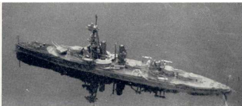
Above: The Airfix Iron Duke is an attractive but realistic subject for motorisation. Here she is afloat but not under way. 'A' turret actuates the switch and is here trained to starboard in the 'off' position.
