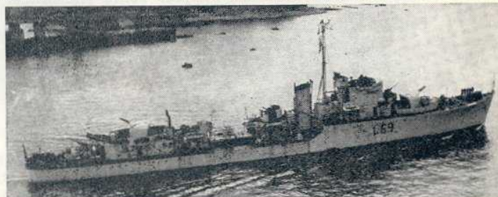
Top: The Leader of the 18th Flotilla, with a black funnel top over one white and one black band; 'X' mounting is trained aft. Above: HMS Tanatside was typical of the Bofors-armed Type IIIs with Carley Floats carried on skids in place of the bridge sponsors. Other Floats are fitted abreast the Emergency Steering Position and one is stowed abaft 'X' gun.
