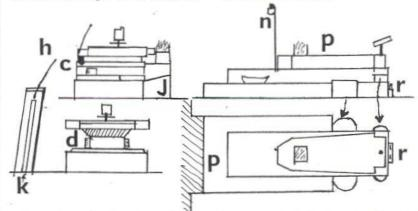
Follow these drawings in conjunction with the corresponding letter keys in the pictures. They give the necessary dimensions for all the modifications illustrated, Mast positions are shaded, also the funnel deck position. In P, the upper deck is taken from the *Tiger* kit, and modified as shown. Note curved wings in after superstructure.
