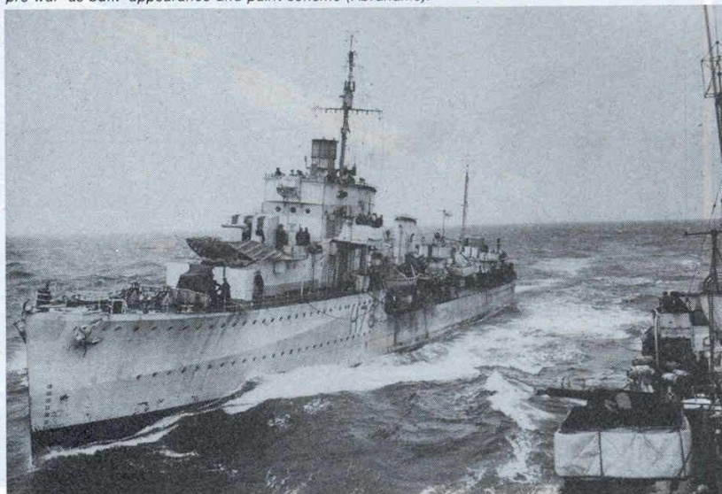
Above: An evocative view of HMS Icarus coming into Scapa Flow. Note the mining rails aft (IWM-A8954). Below: A fine view of Fame as a convoy escort with Hedgehog in 'A' position, cut down after funnel and surface warning radar replacing the gun director (IWM-A13375). Bottom: HMS Acasta shows typical pre-war 'as built' appearance and paint scheme (Abrahams).
