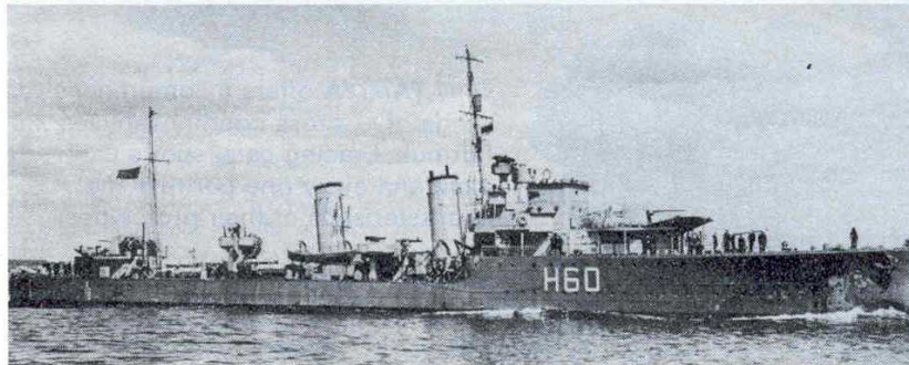
Top: HMS Hesperus with angled front bridge, extra DCs instead of 'Y' gun, stump main mast, and exhaust on fore funnel (IWM-A7101). Above: HMCS Ottawa represents one of the simplest of adaptations from the basic Airfix kit, with attractive colour scheme in light and dark grey (IWM-CAN164).
