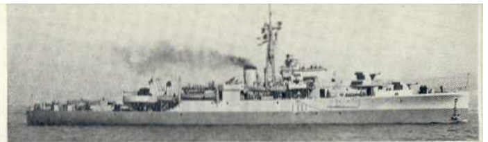
Scotts of Greenock built Lark and Lapwing, which were virtually identical. Lark has a lattice foremast and an all-Oerlikon close range armament in this 1945 photo.
