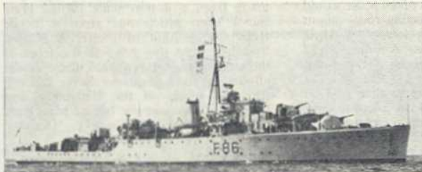
Pelican , off Portsmouth in 1954, re-armed with single Bofors, but retaining her tripod foremast.
