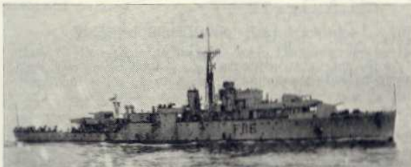
Cygnets features in the variants table. Here, the starboard quad pom-pom is clearly visible abaft the funnel. Notice her tripod foremast and 'crowsnest'. Left: Most famous of the class was Amethyst , here seen returning shell-scarred from the Yangtze action in 1949. Note the 'plugged' shell holes near the waterline.
