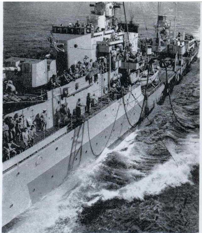
Above: A close view of HMS Rotherham in 1945 as she transfers oil fuel from the carrier Illustrious in the Far East Fleet. Useful details to note are the single Oerlikon mounts in the wings abreast the after radar mast, bridge wings with twin Oerlikons, and the early type of shield on the 4.7 inch guns (Imperial War Museum).
