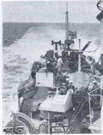
Above: HMS Wager in the Pacific in 1945 with a single Bofors mount and twin Oerlikon mounts abaft the funnel. The Hazemeyer Bofors mount is further aft with its radar aerial just visible above it.
