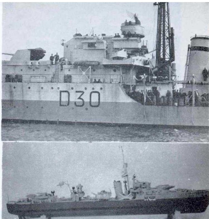
Top: A superb detail view of HMS Wager , 27th Destroyer Flotilla, British Pacific Fleet, in 1945. Note the red/yellow Carley float, the single small director with superimposed radar aerial, twin Oerlikon mount in bridge wing, and later type of shield to 4.7 inch gun (E. W. Elwick). Above: HMS Rocket modelled by Peter Hodges as described in the text.
