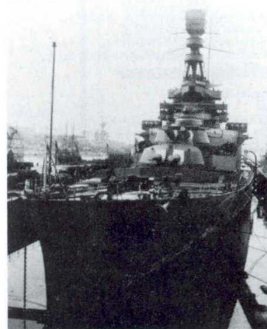
Above: Repulse in 1939 or 1940 leaving port. On the foretop is a new secondary director and an early radar aerial is just visible atop the main mast. One of the new light AA mounts can be seen outboard of the triple 6 inch turret and the end of an electric crane can be seen behind it. A 32ft pulling cutter rigged as the seaboat. Right: Repulse in dock apparently at the time of her 1936 modernisation.
