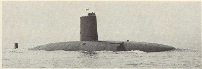
HMS Conqueror, one of the 'Valiant' class SSN's. The 'Valiant' class were the first nuclear powered submarines built of exclusive British design and construction, and had an impressive increase in capabilities over the earlier Anglo/American built Dreadnoughts (S101). Their speed was increased by about 5 knots, and their range was considerably more than the earlier boat (Photo: MoD Navy).
