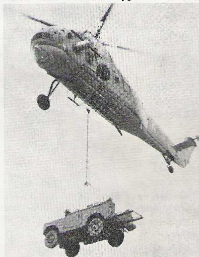
Above: Though landing craft are the main means of ferrying equipment ashore, choppers can also handle light loads. Here a 72 Sqn Wessex lifts a Marines Land Rover WOMBAT carrier. Gun is carried as a second load.
