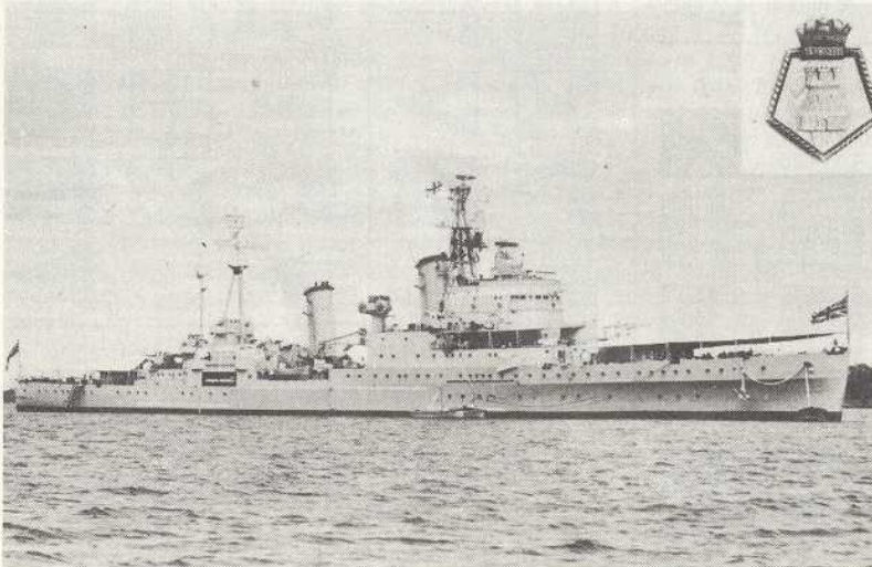
The 'Town' Class cruiser HMS Newcastle, after her post-war modernisation, with an awning spread over the fo'c's'le and a Rear Admiral's Flag flying from the fore topmast. Her hull shows a good example of a 'knuckle bow' (Navy News Photo Series).
