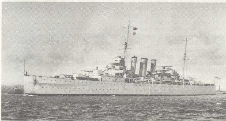
The Airfix Suffolk kit makes conversions to a large number of British 8-inch cruisers possible. This is HMS London in February 1937 flying the old 'Right of Way' hoist. The big radial davits of her boats are clearly visible (Wright & Logan).
