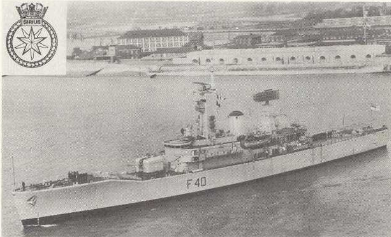
The old gun battery of Fort Blockhouse at the entrance to Portsmouth Harbour forms the background to this photo of the 'Leander' Class frigate Sirius, as she proceeds to sea. Observe the draught marks at the bow — white numbers against the black boot-topping and black against the ship's side grey. She is in the narrow fairway, and flies the Naval 'Right of Way' hoist of the period — International Code Pennant over flags ZV (Navy News Photo Series).
