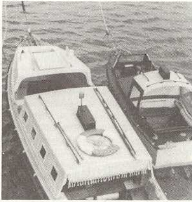
Looking down on the lower boom, rigged to starboard, with the 25 foot motor cutter inboard and the 'skimmer' outboard. Note, in the latter, the driver's cockpit forward and the passengers' compartment aft. Both boats have illuminated ship-name boxes on their canopies.
