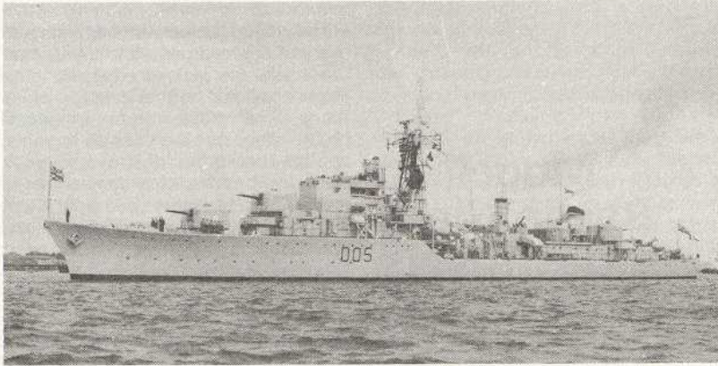
Daring, re-classified as a destroyer, and wearing her pennant numbers in 1959. She is much as modelled in the Airfix kit, but the after set of torpedo tubes has been removed and inflatable liferafts have replaced the original Carley Floats. Note the height of the Jack staff rigged in the bows (Wright & Logan).
