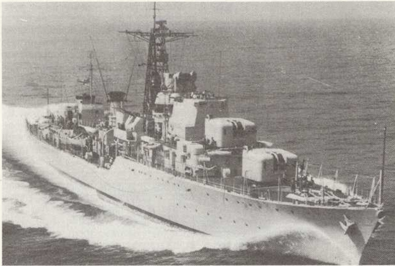
There were many major changes to the 'Daring' Class in the course of their service lives. Here, HMS Daring is seen in Portsmouth Harbour during the late spring of 1967, having been modernised. She has a new director, twin Mk 5 Bofors have replaced the STAAG mountings on the bridge wings and her after superstructure is continuous from 'X' gundeck to the break of the fo'c's'le. This was probably a ceremonial occasion, for she is flying a Union Jack and two White Ensigns whilst under way. Note the large Ensign on the Ensign staff and the smaller one at the sea position at the peak of the gaff (Wright & Logan).
