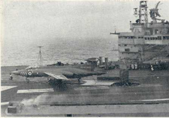
Above Buccaneer S2C of 809 Squadron on the forward catapult. The blast screens are raised immediately behind the aircraft, and the hold-back stop can be seen beneath the tail.
