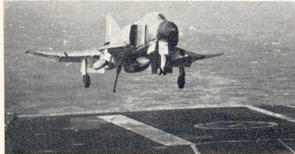
Top Buccaneer S2C about to touch-down on Ark Royal's round down. Practice bombs can be seen on the wing pylons. Above a rocket-armed Phantom FG 1 about to hit the deck. Large flap area is necessary to reduce the speed of this American fighter for landing on small British carriers. Right a Phantom of 892 Squadron is marshalled on to the waist catapult. Towing vehicles can be seen parked by the island structure (Author's photos).
