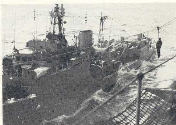
Below jack-stay ship-to-ship transference is regularly practised as a training exercise, as between Ark Royal and HMS Kepple .
