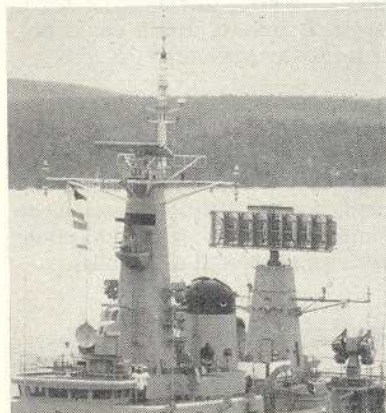
Above top: A typical Leander class frigate, Arethusa has 903 on her director, 976 on the forward face of the foremast, with 993 above and the H|F D|F aerial on the topmast. The shorter mainmast carries 965 with its own co-axial IFF. Above bottom: Close-up of the superstructure on Arethusa.
