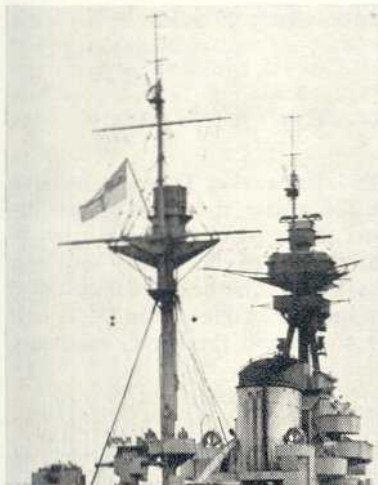
Above top: The battleship Revenge has 285 on both HACS directors, 273 in the mainmast 'lantern' and the double 79 or 279 aerials at each mast-head. Above bottom: Close-up of the two HACS directors on the Revenge .
